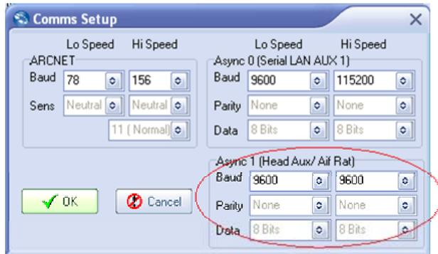
...Check Baud rates on **Async 1 (AUX)** match the device output (default Digiquartz output is 9600 baud).
