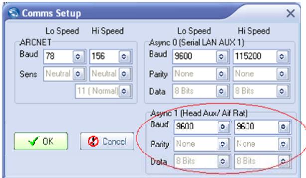
...Check Baud rates on **Async 1 (AUX)** match the device output (PA Altimeter is 9600 baud output).
