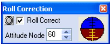
To enable the Attitude Sensor and apply angular corrections to the Profiler data, enable the '**Roll Correct**' check-box.
