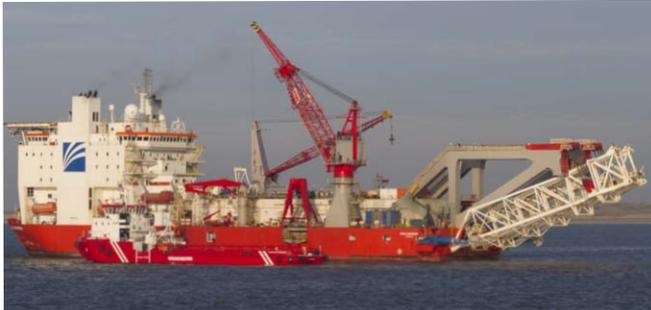
*Pipel-lay vessel with stinger at the rear.*
