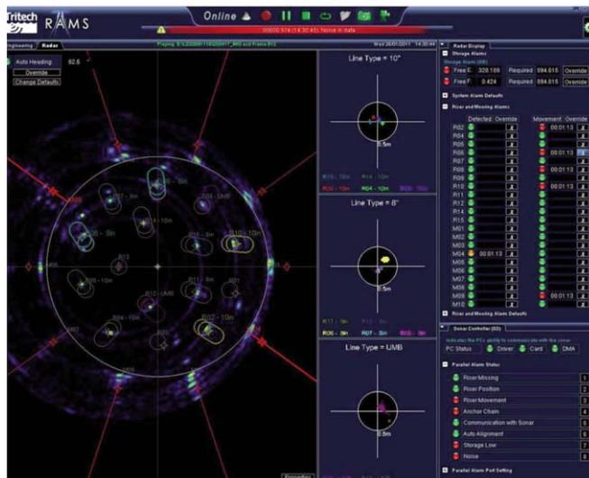
Graphic showing a screen shot from the RAMS™ software showing the real-time imagery of the risers and alarm triggers.
