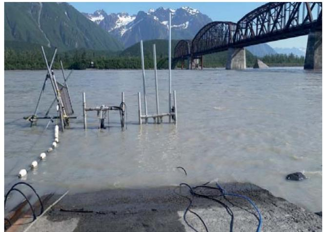
120 degree swathe covered by 256 x 1 degree beams results in an effective angular resolution of 0.5 degrees for images of superb clarity.
